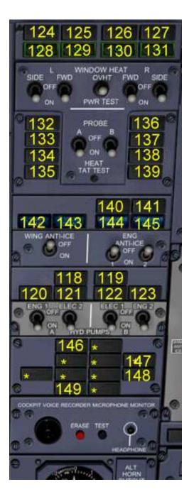
**Note 1. Window Heat:** Window Heat Led's remain On when they are switched On. Overheat Led's remain Off until the Overheat Test Switch is used which in turn illuminates them.
