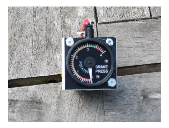
The Brake Pressure gauge made from plasticard, Hitec HS-55 servo, plastic gears and a gauge face courtesy of Juan Cordon . The bezel is made from plastic waste pipe!
