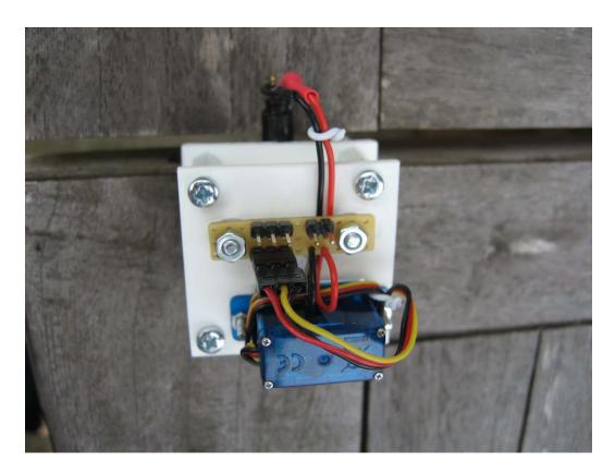
Rear view of the gauge showing the servo, electrical connections and lead to led lighting for the gauge face
