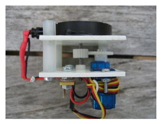
Side view of gauge showing gears and connections between servo and gauge needle
