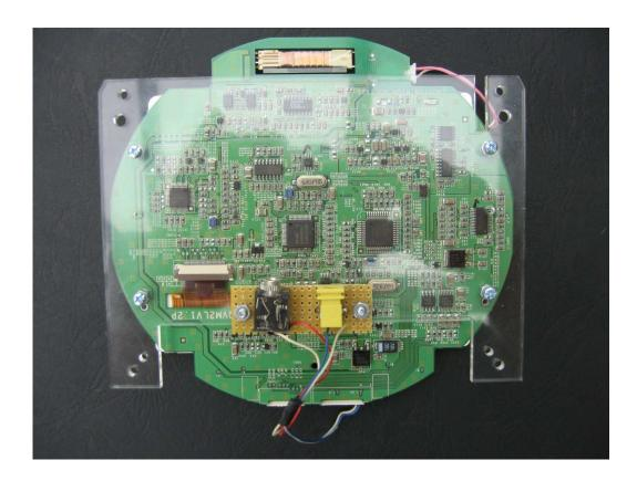
The mounting plate for the composite video and power inputs. There is an excellent article on the FDS site in the Tutorial section which explains how to dismantle the PSOne screen and remove the redundant wiring
