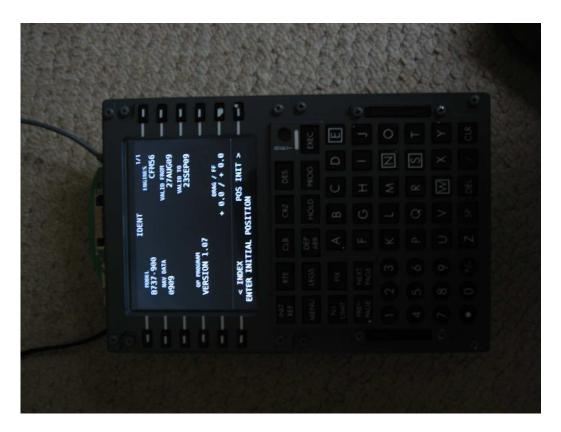
This output screen is running at 1024 by 768 under composite video. There are many articles suggesting how to convert the PSOne to run on VGA but it is far from straightforward and requires a video board with special timing facility – I am happy with the quality of the composite output.
