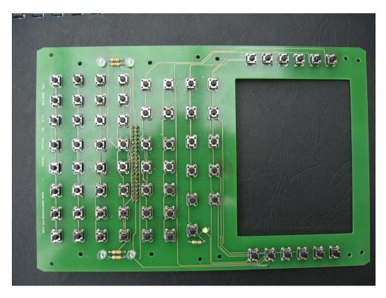
The assembled keys – a few need the paint retouching where I managed to cause some damage
