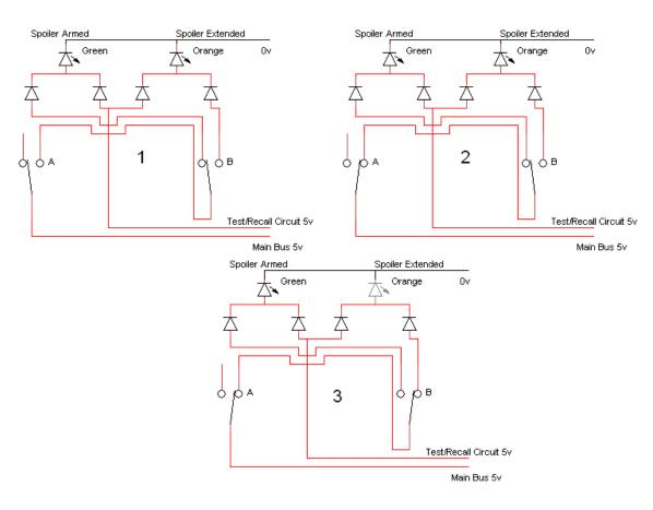
The two switches are A, the control switch and B, the director Switch. Switch A basically turns the power on and off and switch B directs it to the correct LED based on the position of the lever.
