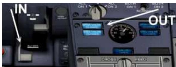
What this does is switch the relay when the Idle/Cut Off Lever is set to Cutoff. I am forever grateful to Peter Dowson for pointing this out to me and to Paolo at CPFlight for teaching me how to get the lines written for the DigitalOut.cfg file.
