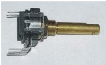
This is the CTS288 Rotary Encoder c/w 'Push to Make' Switch. They are available from the Opencockpits shop at [www.opencockpits.com](http://www.opencockpits.com). They are relatively inexpensive, nice quality and robust. This is exactly how they work. If you look at the drawing below of the CTS288, it has 5 connector pins, a set of two which are the push to make switch and a set of three which are the encoder contacts. These are labelled A, B & C with C being the common.
