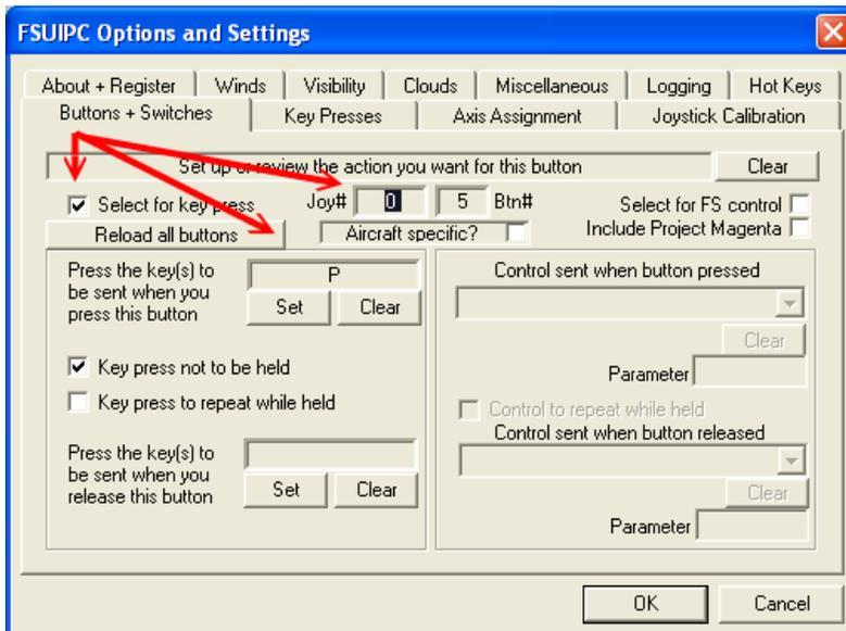
Check the Select for key press box and in the box below set the key to be sent when you operate that component. Now systematically work your way across the switches (remember there's 25) until you have assigned all the keys to each input that correspond with your PMDG Key Command Assignments.
