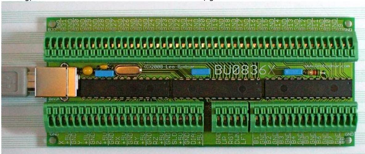
Every input on this card is independent, so using the X board, there is no more working out which row/column is which button and where the diodes go. But my original diagram does not help people deciding to build using the X board and I have had several mails asking me to help. So here we go.....
