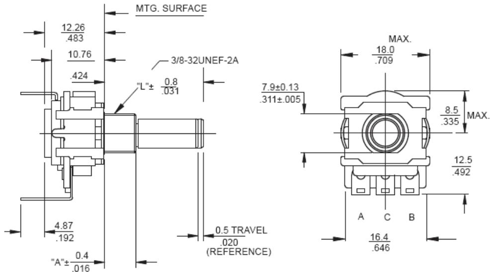
Remember the A, B and C relationship because we are going to use that when connecting up to the BU0836 joystick controller. The 'push to make' switch can be connected any way round because it's just a simple contact switch.
