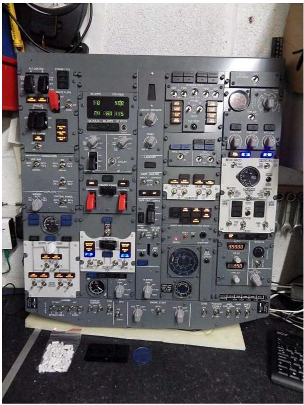
Brand New Simworld Overhead Panel FOR SALE. This is one I built earlier in the year for Andrew who unfortunately owing to incapacitation is having to sell off his sim. Unit is wired to 3 x BBI-32 Input Cards and 2 x Phidgets LED64 Output Cards. There is also a POLOLU 6 channel Servo Controller onboard to control the working APU Gauge. Contact Andrew <a href="mailto:pringleno1@hotmail.com">pringleno1@hotmail.com</a>
