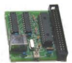
My Keyboard Emulator has it's own .ini file which I can modify with a standard text editor. It plugs into a spare USB slot on my computer which recognises it as a USB keyboard....so far so good. Communication with the card is via a standard 40 wire IDE lead (same as from your Hard Drive to your Motherboard – you know the type). It has a connection Matrix using 11 Letters and 8 Numbers. So
