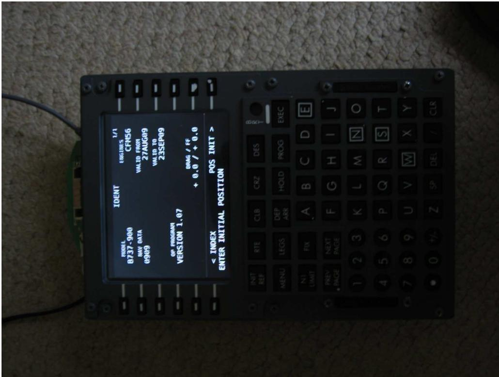
This output screen is running at 1024 by 768 under composite video. There are many articles suggesting how to convert the PSOne to run on VGA but it is far from straightforward and requires a video board with special timing facility – I am happy with the quality of the composite output.
