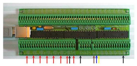
Red Arrows are 5vdc for LED Black Arrows are GND For LED Blue Arrow is Common GND For Switches Brown & Yellow Arrows are Any Button Inputs for Microswitches.
