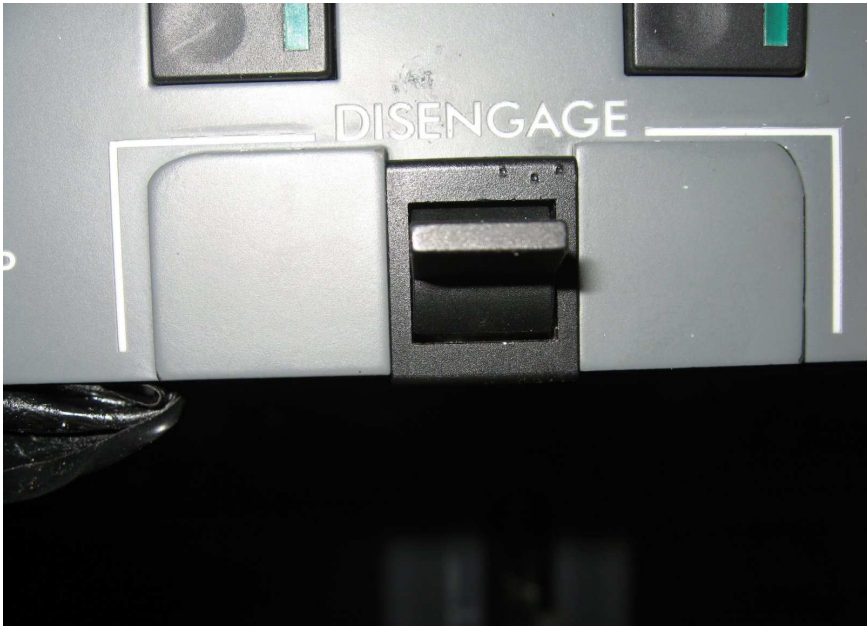
A/P switch before dismantling showing black collar surround to switch
