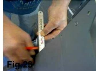
When you are completely satisfied that the sidewall is correctly placed, mark a pencil line on the sidewall block as in Fig.21. Take the dimension from the rear of the sidewall block to the edge of the sidewall panel itself shown in Fig.22. Transfer this dimension to the other side. This ensures that your covers will fit evenly and 'square'.
