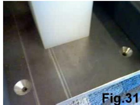
**Note:** At this point, you may like to think about fixing your Pedals. Although access to the rear fixing screws is possible with the covers fitted, the front fixing holes are enclosed. So, now would be a good time to put your Rudders in place to mark up and drill the final fixing holes.
