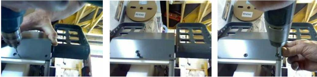
All that remains is to fix the front Lower Panel in place. There two options here. Drilling and screwing in place or using Contact Adhesive. Whatever you choose, please bear in mind that this panel needs to be fixed last of all after you have secured the front fixings.
