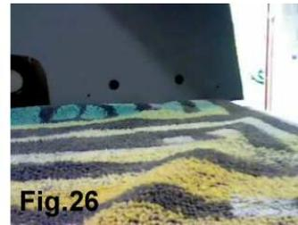
Remove the outer sidewall panel and with the inner panel correctly in place, mark two holes both fore and aft of the lower cutout in the panel. Use a dimension of 25 – 30mm as shown in Fig.24. Make sure you avoid the pilot holes we drilled earlier. Drill and countersink the 4 holes each side and fix the inner sidewall to the sideblock as in Fig.26.
