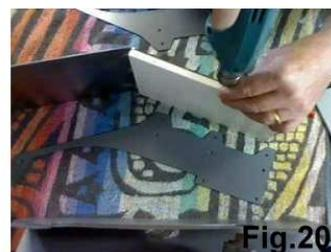
**Note:** Now you have the major parts assembled, at this point we recommend that you have a 'Practise Assembly', so you understand how the components fit together. With the panels correctly placed in relation to each other, we will also prepare for final fitting by marking up the position of the side panels in relation to the baseplate.
