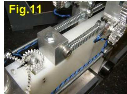
Once the springs have been attached to the Lever Arm, we then have to stretch the springs and bolt them to the anchor block as shown in Fig.11.
