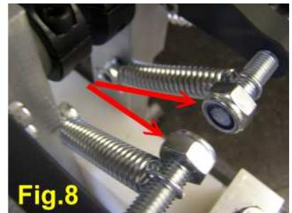
Using a 17mm spanner remove the two Nylok nuts as indicated in Fig.8 on the end of the end of the Fulcrum Lever spring anchor bolts.
