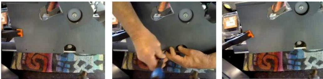
Place the top cover in place making sure that it fits neatly at all the four contact points at the rear and front of the sidewall panel. Using eight of the small screws supplied, fix the top cover to the sidewall panel front and back, both sides.
