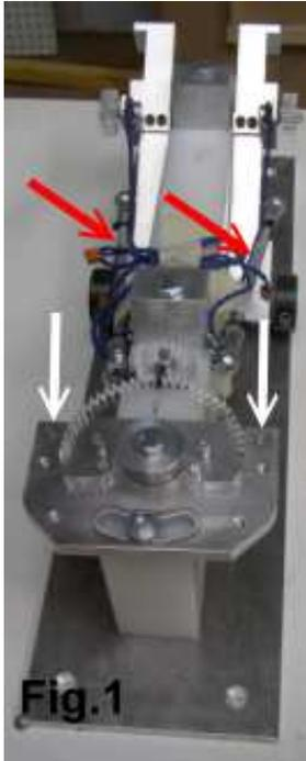
**Step 1. Attaching the Rudder Pedal Lever Arm Rods.**
