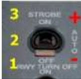
Now looking at the switch on the left (from the Airbus), to get from position 1 (Off) to position 3 (On), two inputs are required. And to get from the On position to the Off position, again two inputs are needed. To switch from Off or On to Auto, only one input is required, but they all must be in the correct direction.
