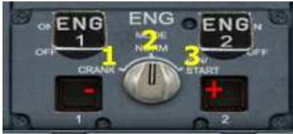
Then another application springs to mind. A 3 position rotary. Good example is the Engine Mode Switch on the A320.
