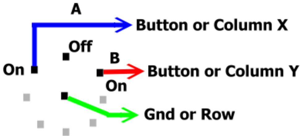
Result is a directional 3 way switch which inputs to Button X at each movement one way and Button Y at each movement the other way. So it's off to FSUIPC and record the macro's :o))
