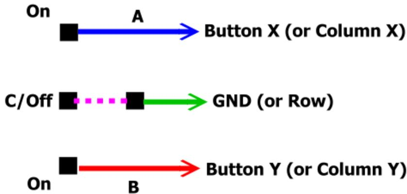
Looking at the above diagram of a 3 position (centre off) switch, it's possible to replicate the position 4, 5 & 6 switch states in the truth table.
