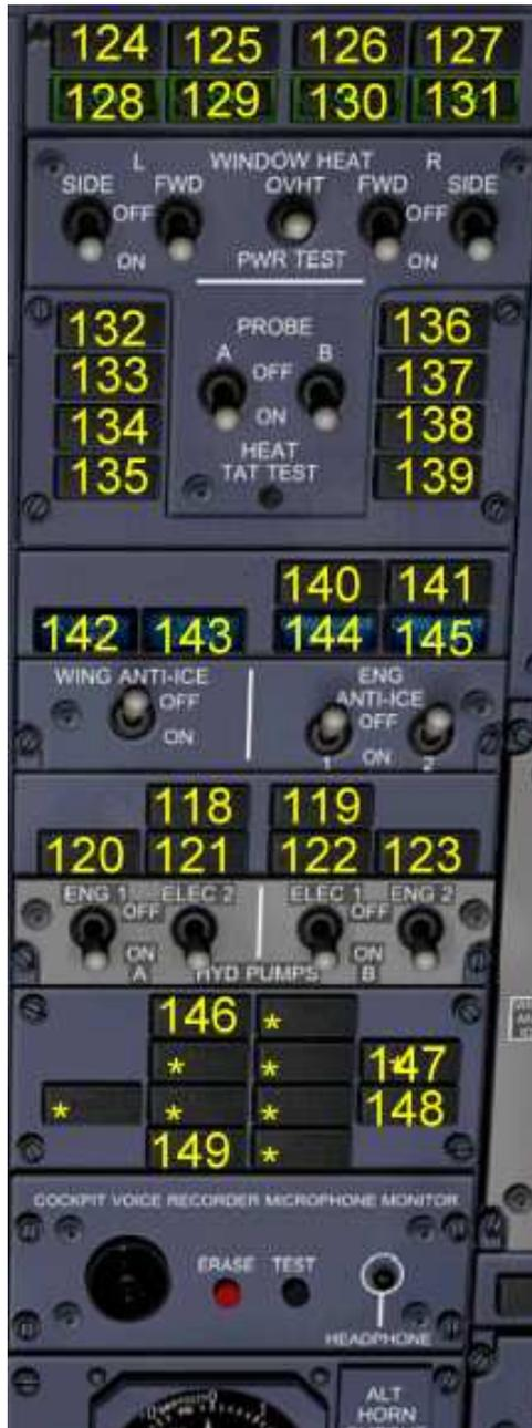
**Note 1. Window Heat:** Window Heat Led's remain On when they are switched On. Overheat Led's remain Off until the Overheat Test Switch is used which in turn illuminates them.
